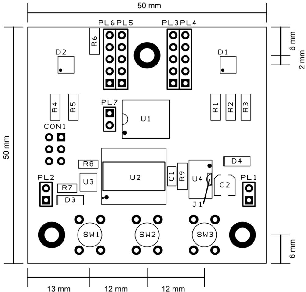
NOTE: Assemble CON1 on bottom side.
